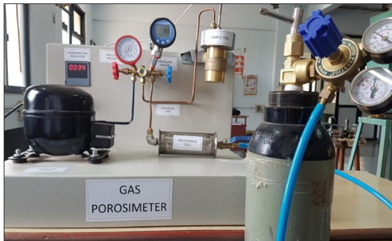
Figure 3. Gas porosimeter setup to measure the grain volume of bone scaffold
